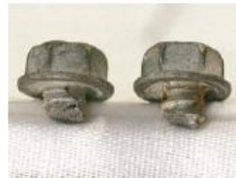
410 fastener with aluminum-filled topcoat
