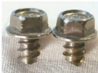
Modified 400 series SS fastener
