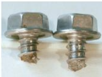
410 SS super passivated fastener with plain finish
